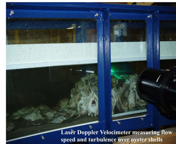
Laser Doppler Velocimeter measuring flow speed and turbulence over oyster shells
